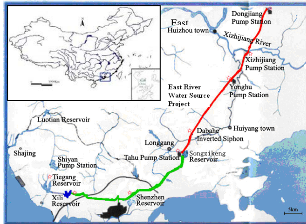
Figure 1 Layout of the tunnels of East River Water Source Project: red line - water transfer tunnels, green line - water deliver tunnels
