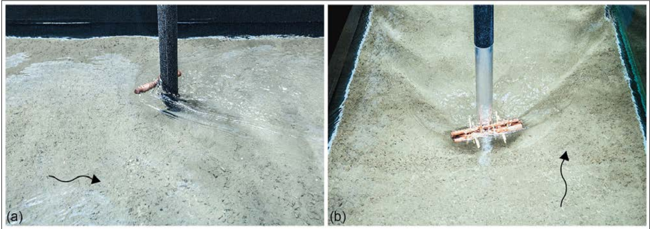
Figure 7. (a) Side view of LW accumulation with a rough bridge pier (Test C3), and (b) plan view of LW accumulation for congested logs with 3D branches (Test E8).
