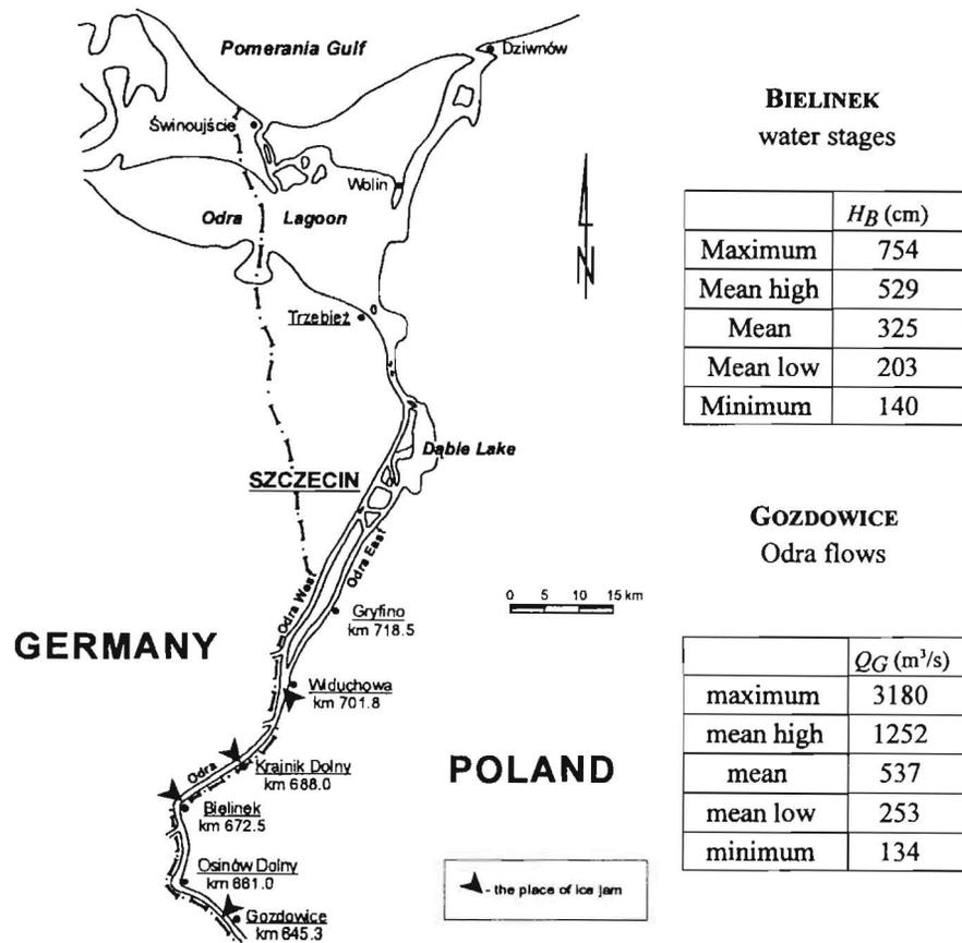
**Fig.1.** Situation scheme of lower Odra, characteristic water stages in Bielinek (1949-1999) and flows in Odra at Gozdowice cross-section (1952-1999)
