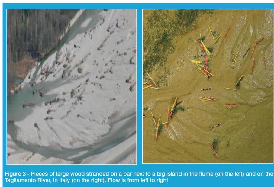
Figure 3 - Pieces of large wood stranded on a bar next to a big island in the flume (on the left) and on the Tagliamento River, in Italy (on the right). Flow is from left to right
