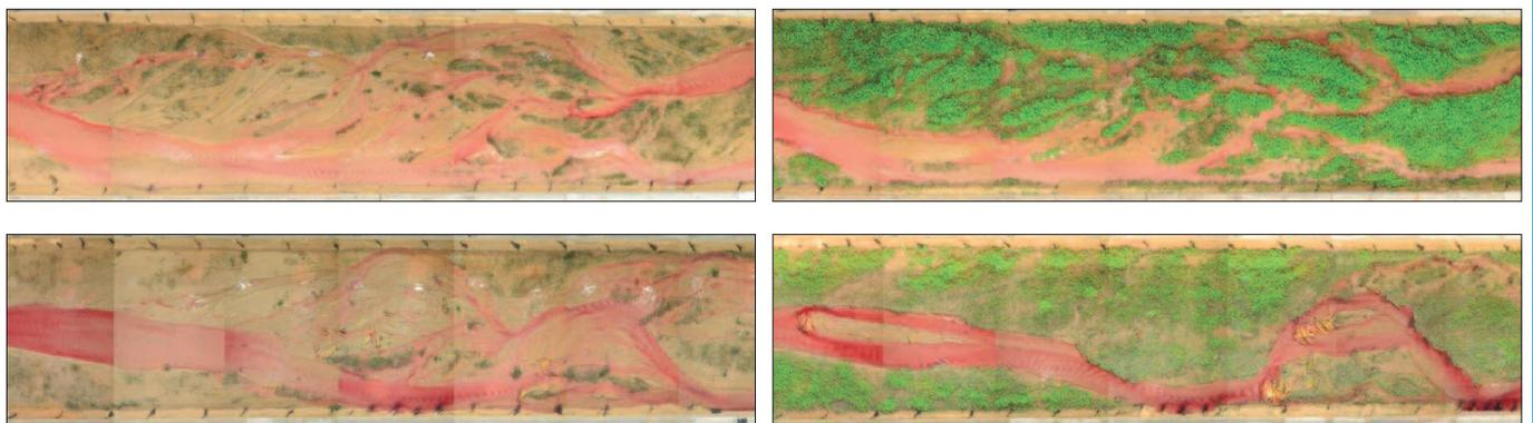
Figure 2 - Vertical photos of two flume channels with self-formed braided pattern taken a few days after the alfalfa seeding (on the left), and towards the end of the experiments (on the right). Photos refer to the flume channel where only alfalfa was seeded but no logs were fed into the system (above), and to the flume channel where logs were also fed at a rate of 120 logs h<sup>-1</sup>. Flow is from left to right.
