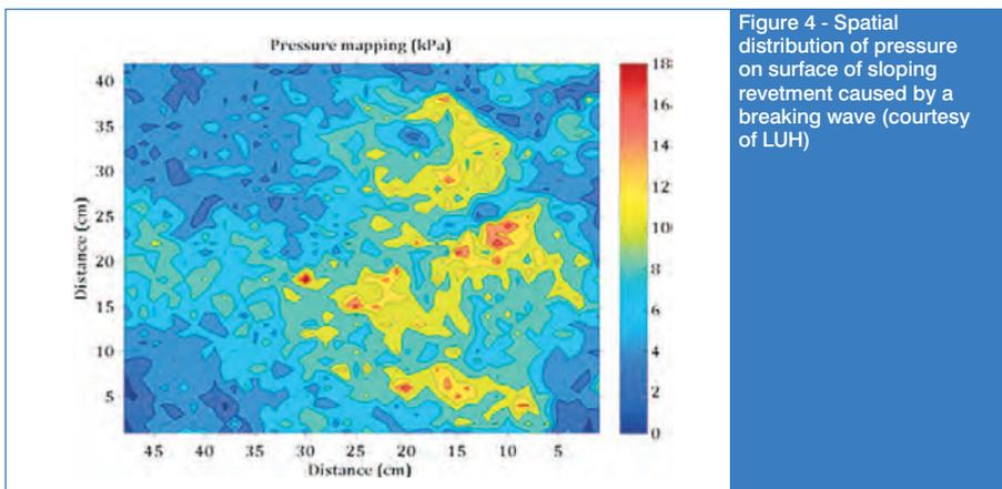
Figure 4 - Spatial distribution of pressure on surface of sloping revetment caused by a breaking wave (courtesy of LUH)
