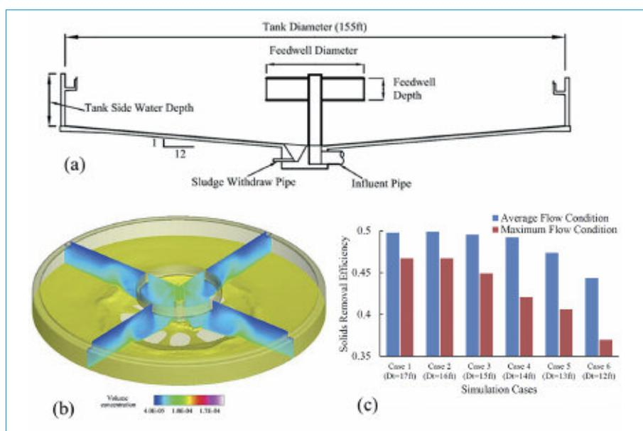
Figure 1. (a) Schematic of the primary settling tank; (b) volume concentration distribution in the tank; (c) solids removal efficiencies of different tanks under average and maximum flow conditions for different tank depths (D<sub>t</sub>) (from Liu and Garcia, 2011. Reprinted with permission of ASCE)
