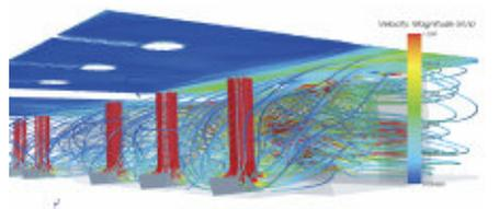
Figure 4. Pumps inlet at pump station. Flow rate: 5 m³/s, distributed through 5 submersible pumps. Flow pattern shown through streamlines to assess admission requirements for safe pump operation
