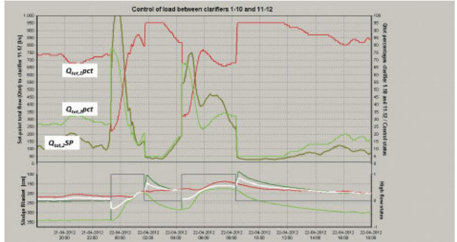
Figure 8. Marselisborg WWTP – sludge storage control using a virtual sludge blanket. Bottom: SB<sub>Avg,1</sub>: red; SB<sub>Avg,2</sub>: light green; SB<sub>Avg,2-virtual</sub>: green; SB<sub>Avg,WWTP</sub>: white
