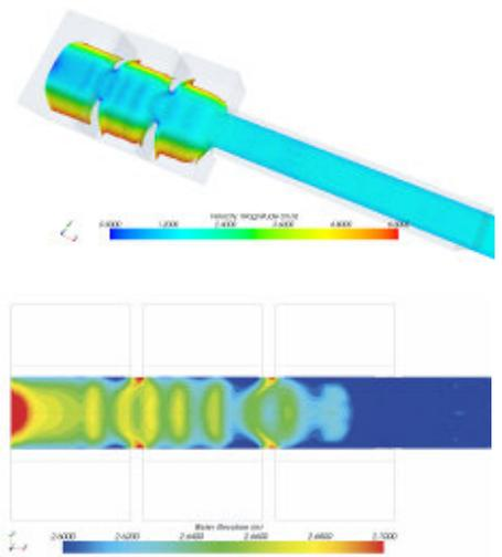
Figure 3. Water approaching through open channel (channel width: 2.5 m; flow rate: 6.5 m³/s). Velocity distribution in impinging flow at closed extremity composes non-uniformity in the flow caused by lateral discharge weirs. Lower image displays free-surface height relative to datum
