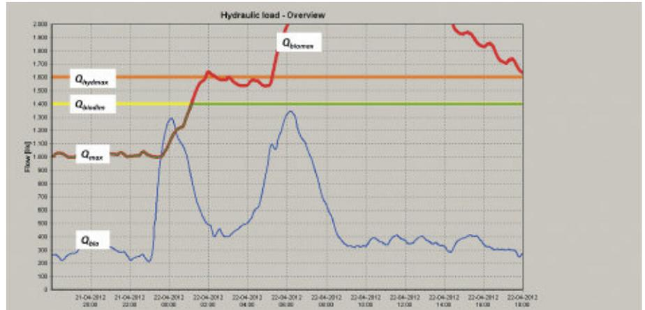
Figure 9. Marselisborg WWTP – maximum hydraulic load,  $Q_{max}$
