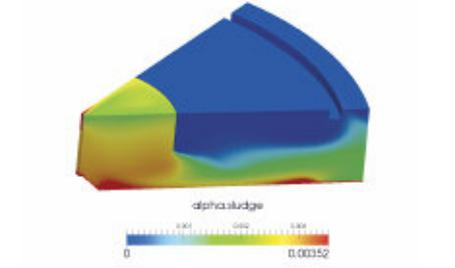
Figure 6. Secondary clarifier (18m radius) sludge blanket modelling. Flow rate ~1.2 m³/s. Colours represent sludge concentration
