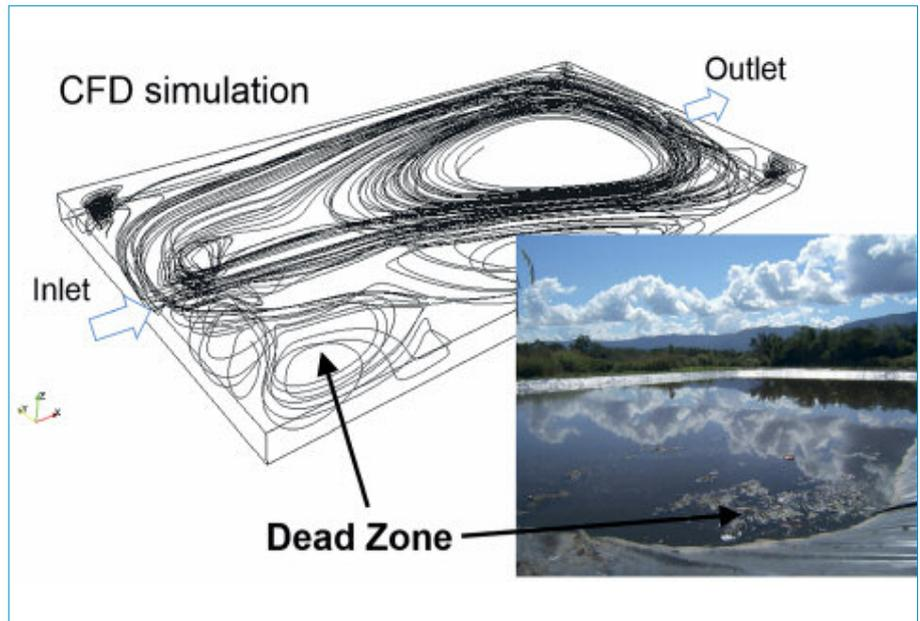
Figure 2. Dead zone in a wastewater stabilization pond, San Antonio, Bolivia modeled in Verbyla et al. (2013)
