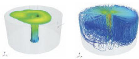
Figure 9. Central injection gas based mixing. Gas volume fraction iso-surface and streamlines coloured by velocity magnitude
