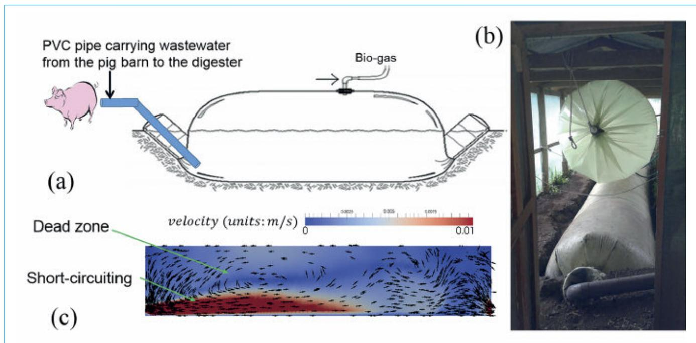
Figure 3. (a) Schematic, (b) photo, and (c) simulated internal flow of the anaerobic digester in Costa Rica studied by Kinyua et al. (2015)
