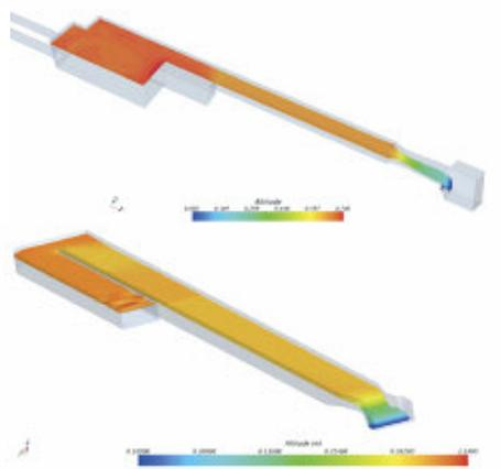
Figure 5. Flumes operating under the influence of discharge chamber and channel bend. Flow rates approximately 1 m³/s
