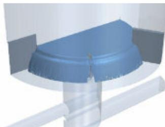
Figure 2. Discharge weir with water injection at the bottom (Diameter: 8 m; flow rate: 4 m<sup>3</sup>/s). This injection pattern gives rise to non-uniform flow distribution across the weirs since the flow is not guaranteed to be symmetrical
