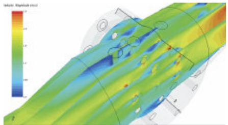
Figure 10. In-line UV reactor with lamps placed perpendicularly to the fluid flow. The intensity of the germicidal irradiation is computed throughout the domain and its eventual absorption monitored through particles released in the flow
