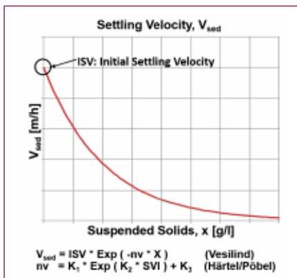
Figure 2. Sludge settling Velocity,  $V_{sed}$
