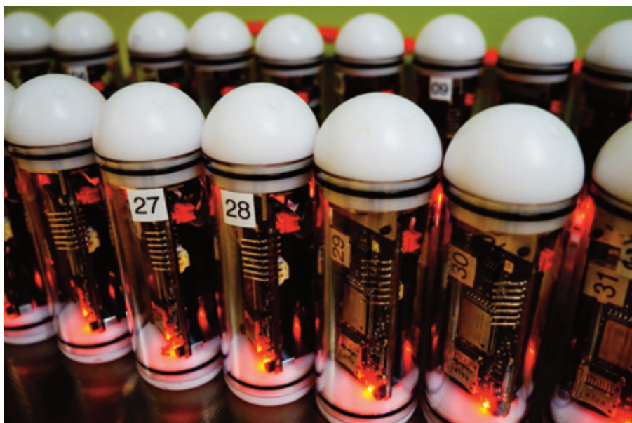
Figure 6. Calibration of the BDS sensors in the laboratory © Jeffrey Tuhtan, TUT.
