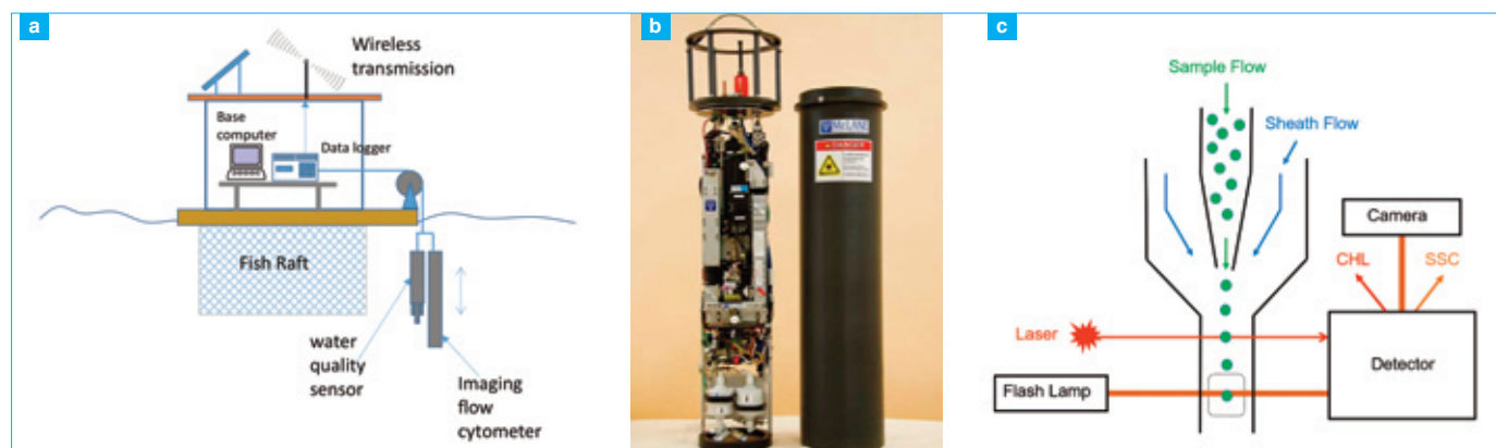
Figure 8. HAB species monitoring at fish culture zone using Imaging Flow CytoBot (IFCB). (a) Field deployment of IFCB at fish raft. (b) IFCB (c) Hydrodynamic focusing.
