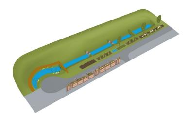
Figure 5: Illustration of the swales, lysimeters and in-ground bioretention cells.
