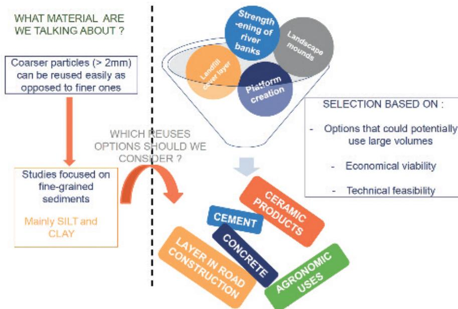
Figure 1. Illustration of potential reuses of dredged fine material disposed on landfill<sup>[4]</sup>
