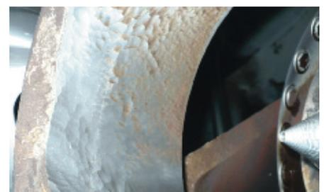
Figure 5. Nozzle wear of the El Canadá HPP turbine due to abrasive sediment particles (Source: El Canadá HPP)
