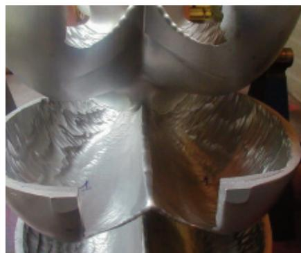
Figure 5. Abrasion on Pelton runner (source: EDF)
