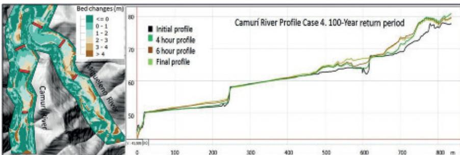
Figure 4. Results for Case 4- Sedimentation upstream of the dams due to a 100-year return period debris flow. The time evolution of the longitudinal bed profile is also shown
