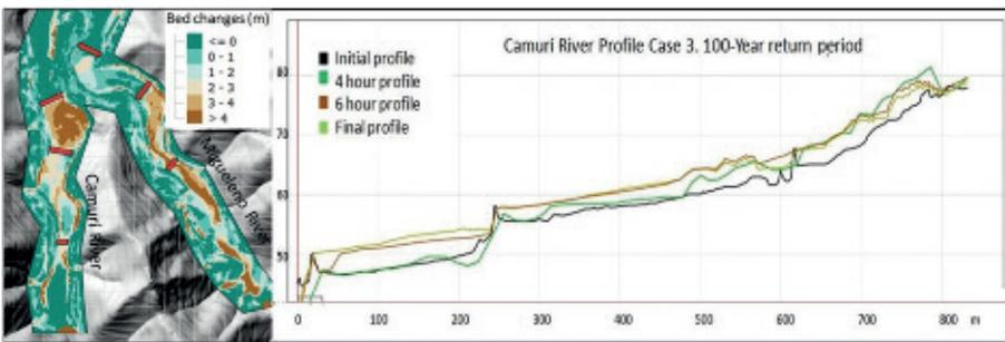
Figure 3. Results for Case 3- Sedimentation upstream of the dams due to a 100-year return period debris flow. The time evolution of the longitudinal bed profile is also shown. The flow pic discharge occurred at hour 5
