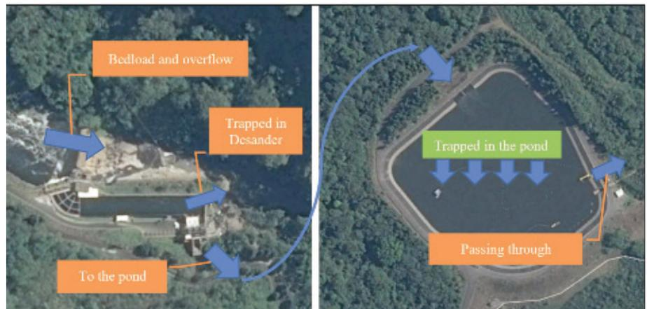
Figure 6. Distribution of sediment load at the headworks (left) and the pond (right) of El Canadá HPP
