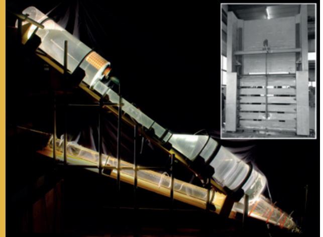
Figure 9. Gondo HPP power and flexibility increase. Physical-scale modeling (big picture) was performed to validate the design of the grid throttle (prototype under construction) placed at the bottom of the lower chamber of the existing surge tank.
