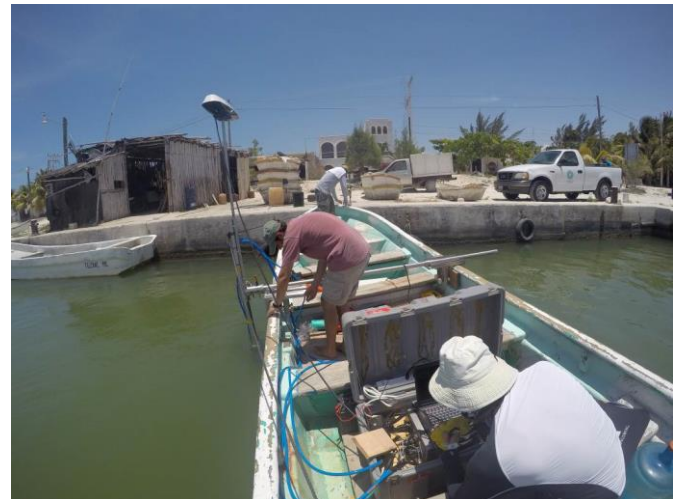
Figure 9: Setting up the shallow water multi-beam.
