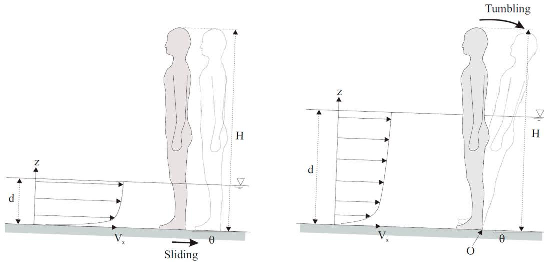
Figure 1. Definition sketch of forces acting on a stationary individual in floodwaters.
