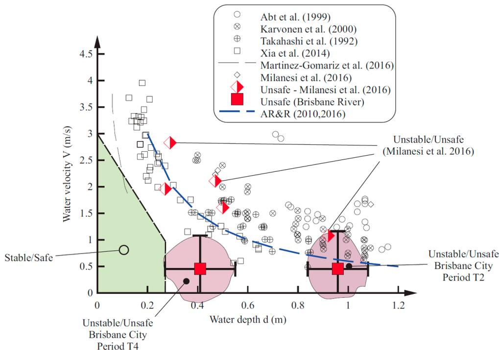
**Figure 5.** Relationship between water velocity and water depth for stability of human body in floodwaters. Comparison between field observations deemed unsafe for evacuation (Red symbols), full-scale tests with adults [11,18,19,23], model data of [14], current guidelines ([13,34] {Low hazard}) and new guidelines (Equation (2)). Scatter bars show the range of instantaneous velocity and water depth measurements.
