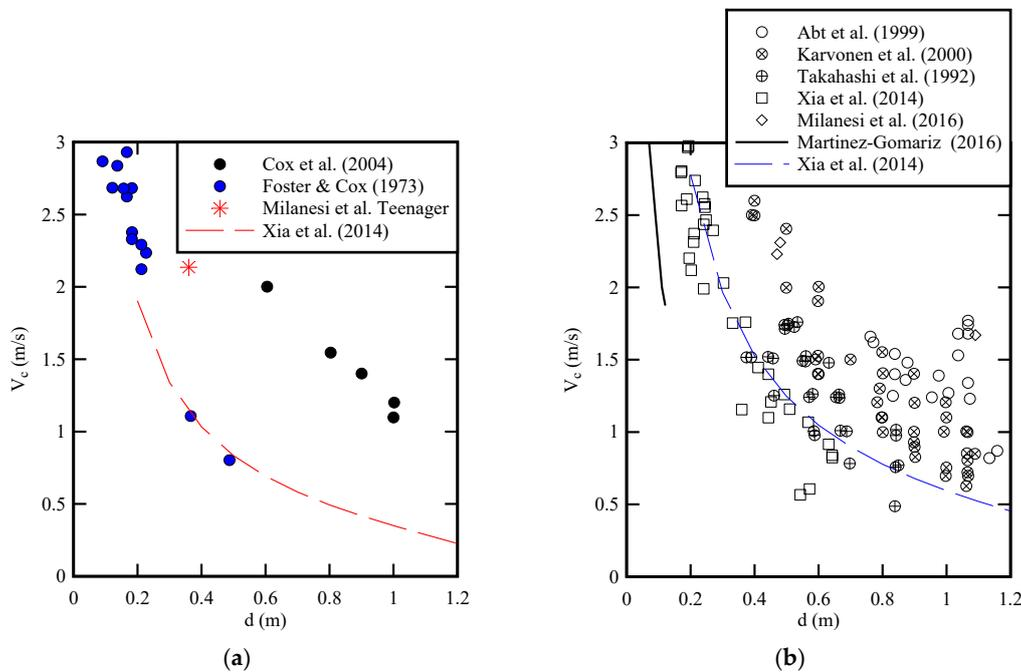
Figure 2. Relationship between characteristic flow velocity and water depth for stability of (a) children and (b) adults. Comparison between field data [27], full-scale tests [11,17–19,23], scaled model data of [12], and semi-analytical relationship proposed by [12].
