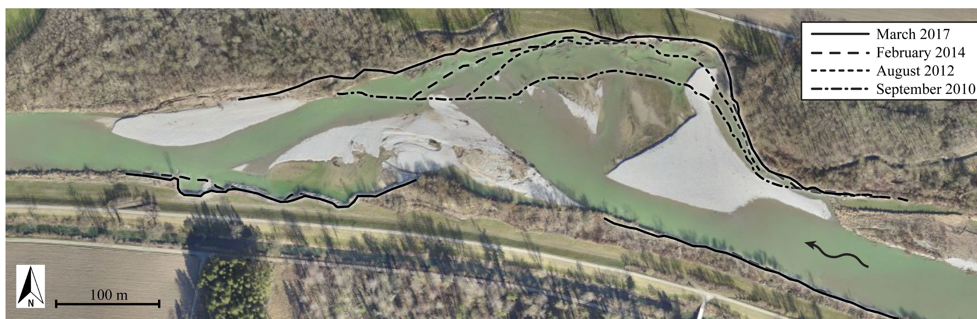
Fig. 1. Lower part of the 1700 m long dynamic river widening Schaffäuli along the Swiss Thur River in 2016. The channel with a former width of 50 m was initially widened in 2003 and has eroded 26000 m 2 of land until 2015 (Orthophoto and data: geotopo ag (Breitensteinstrasse 16, CH-8501 Frauenfeld, www.geotopo.ch)).
