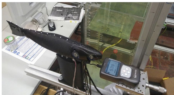
Figure 3: Prototype of the self-propelled active sensor probe [12].
