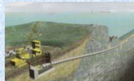
Schematic of a jacked outfall from a cliff top (Courtesy Herrenknecht AG)
