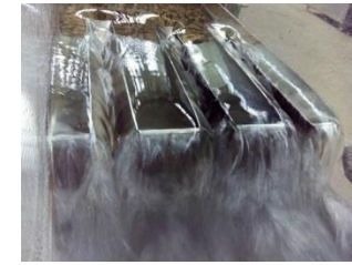
Labyrinth and piano key weirs POLILAB
