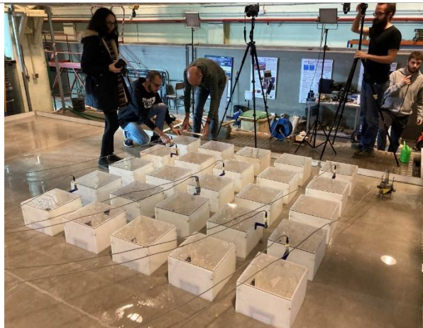
Setting up a scale model of building blocks to study urban flooding considering building basement storage in the STREET facility in the university of A Coruna.
