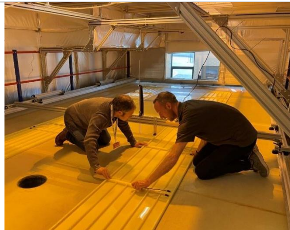
Setting up a model street to study contaminant spreading in urban flood waters, at the above-below ground flume at Sheffield University
