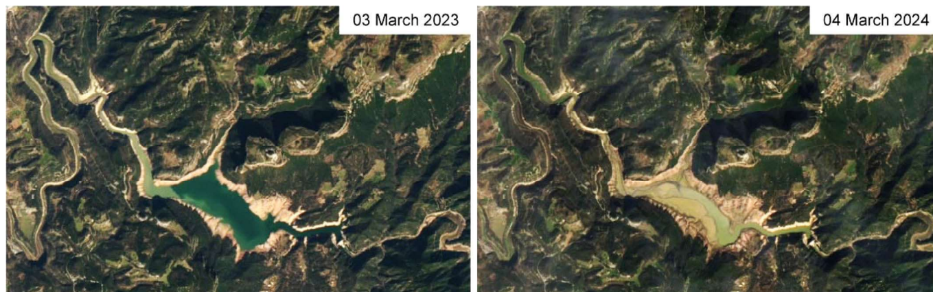
Figure 4 | After three years of drought in northeastern Spain, the stored volume in Sau reservoir was only 16% of its capacity (150 hm 3 ) in March 2024. This is one of the three reservoirs in Catalonia, Spain (Sau, Susqueda and El Pastoral) built in the Ter River which are part of the water supply system for the metropolitan area of Barcelona. Source: NASA.
