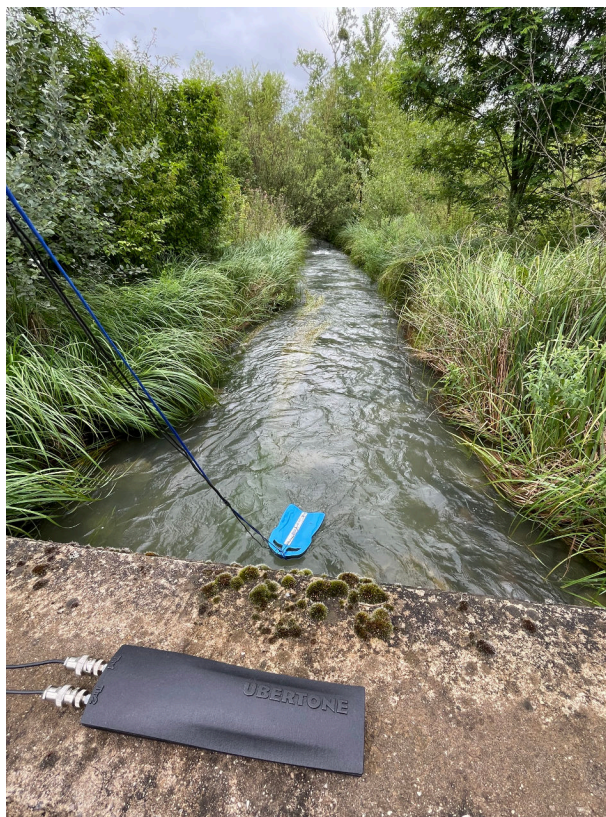
Field measurements: UVP on the fish path
